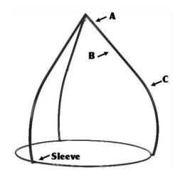
3. For the base, slide one curved base pole through the sleeve on the bottom of the arms, connect a second base pole and place mid-sized silver screw through the lined-up holes of all 3 pieces. Secure with nut.
